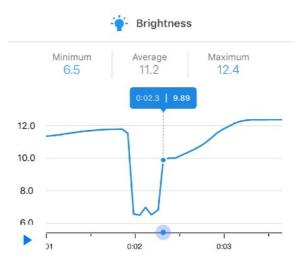
The x-axis shows time in minutes:seconds [min:s] and the y-axis is light intensity in lux.
