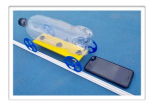
In this measurement we use the **light sensor** of the mobile phone and a light source (lamp or sunlight). Simply start the light intensity recording on the phone and place the phone **face-up** next to the car track. OneCar has enough clearance to move over the phone while the phone is recording the light levels. The resultant graph on your phone should be similar to this:
